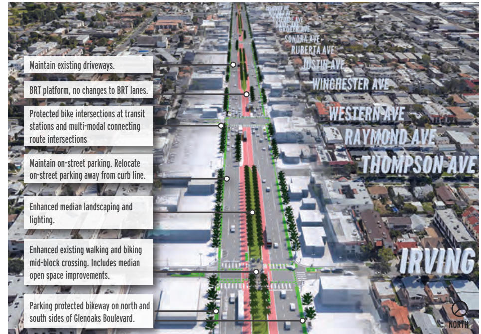
FIG 2.13 TYPICAL PARKING LANE PROTECTED BIKE LANE
